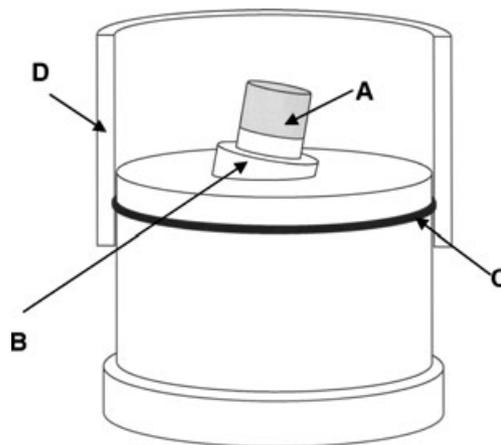
Fig. 3. Jig used for pre-loading and loading tests. A, Norm crown mounted in the jig; B, Brass foundation; C, Rubber gasket and D, Brass cylinder for water storage (shown cross-sectioned).
