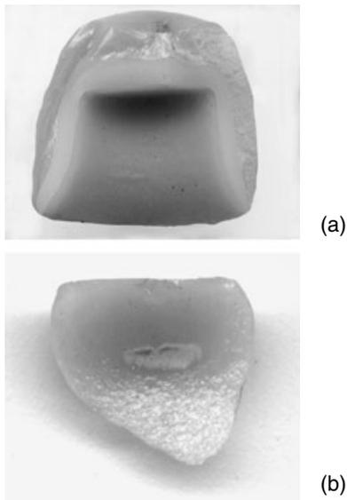
**Fig. 4.** (a) Illustrates a total fracture of an alumina crown where the fracture surface is clearly visible through both core and veneer materials. (b) Illustrates a chip-off fracture of a zirconia crown. The opaque area in the centre of the fracture surface is a part of the porcelain liner.
