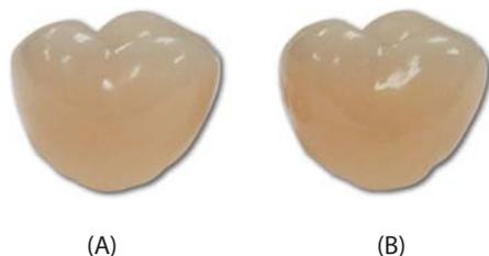
same zirconia, same color liquid, sintered in different sintering ovens
