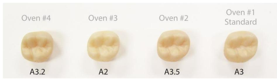
Four different sintering ovens (identical models from the same manufacturer) produced different shade results from the same zirconia disc. This is due to the different PT (performance temperature) of each oven even though the four ovens have the same ST (set temperature).
